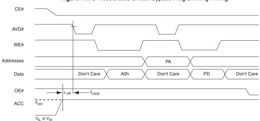
Figure 11.18 Accelerated Unlock Bypass Programming Timing
