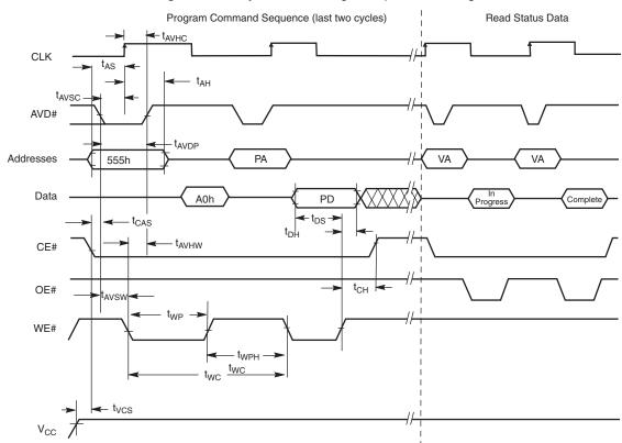
Figure 11.16 Synchronous Program Operation Timings
