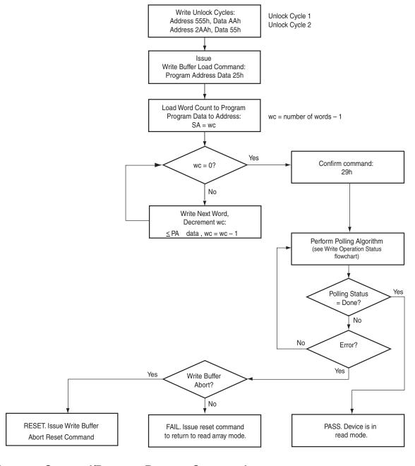
Figure 7.4 Write Buffer Programming Operation
