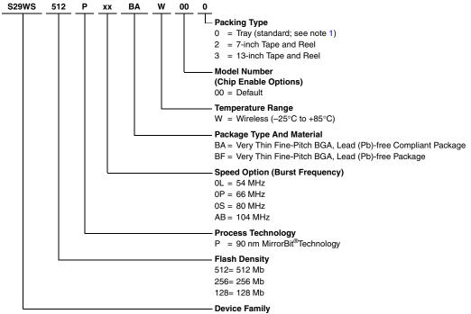
S29WS =1.8 Volt-only Simultaneous Read/Write, Burst Mode Flash Memory
