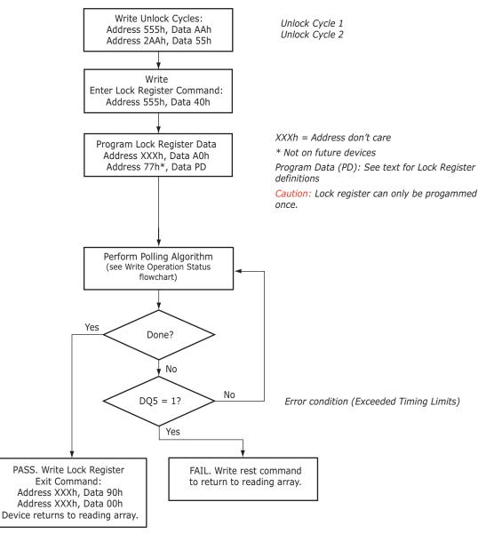
Figure 8.3 Lock Register Program Algorithm
