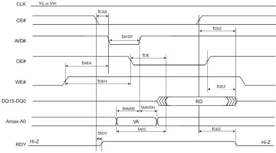
Figure 11.11 Asynchronous Read Mode (AVD# Toggling - Case 3)
