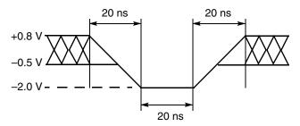
Figure 11.2 Maximum Positive Overshoot Waveform
