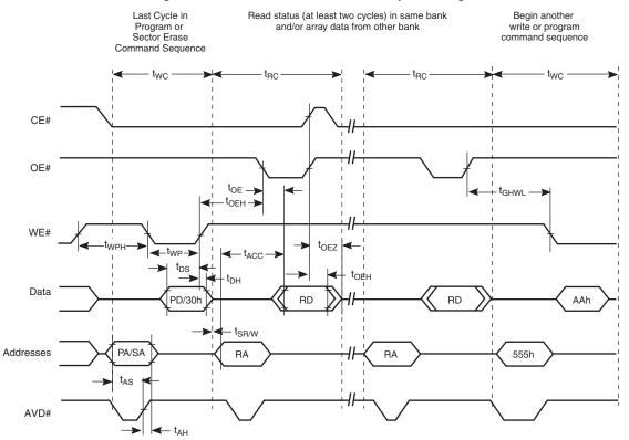
Breakpoints in waveforms indicate that system may alternately read array data from the non-busy bank while checking the status of the program or erase operation in the busy bank. The system should read status twice to ensure valid information.
