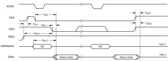
Figure 11.20 Toggle Bit Timings (During Embedded Algorithm)
