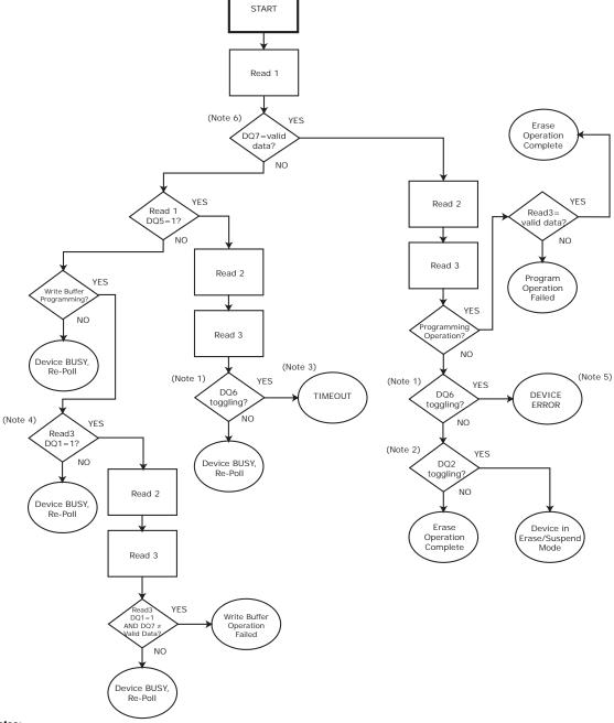
Figure 7.6 Write Operation Status Flowchart
