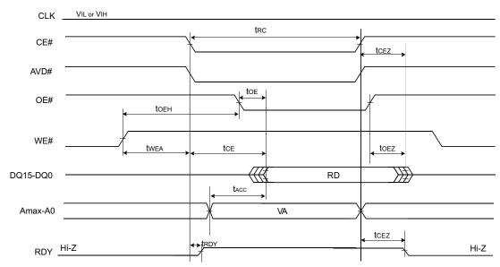
Figure 11.12 Asynchronous Read Mode (AVD# tied to CE#)
